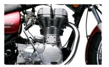
Unit Construction Engine
