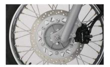
Brake (280MM Disc - Front Brake 150mm Disc - Rear Brake)
