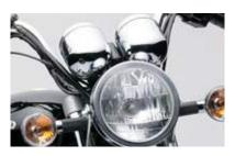
MFR (Multi Focal Reflector) Light with Clear Lens
