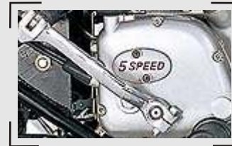
5 Speed Gear box With Left Foot Gear Shift
